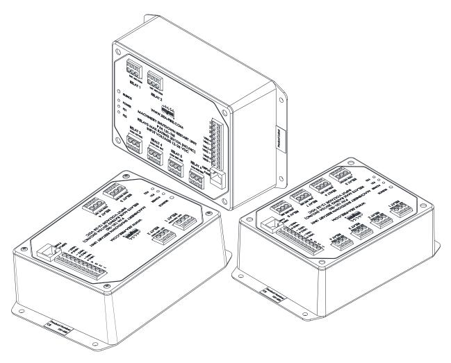
**Warning**: This Sea-Fire Machinery Shutdown Restart System has been designed and tested for use with Sea-Fire automatic and manual Fire Suppression Systems. Installation must be accomplished by or under the supervision of a qualified marine electrician who is familiar with American Boat and Yacht Council (ABYC) or other recognized and accepted marine standards and practices.
