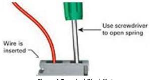
Figure 1 Terminal Block Slot
